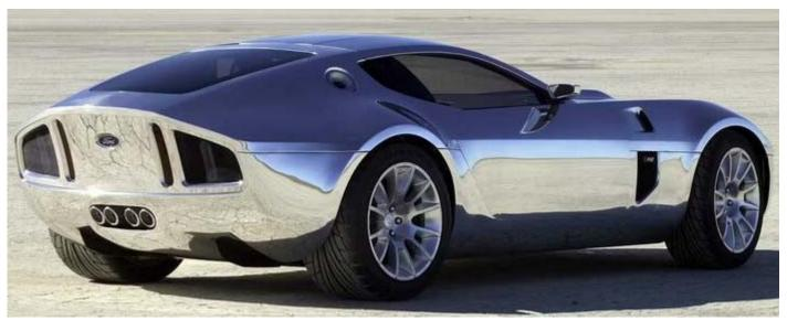
based—needed to be lengthened, too. The GR-1 was not a light car, either, with the concept weighing in at 3900 lb. Ford's target production weight was 3500 lb, and consideration was given to replacing the GR-1's V-10 with a V-8 to achieve that goal.
