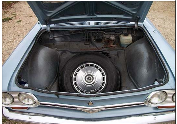
Because of the AC unit, the spare tire is relocated to the front trunk
