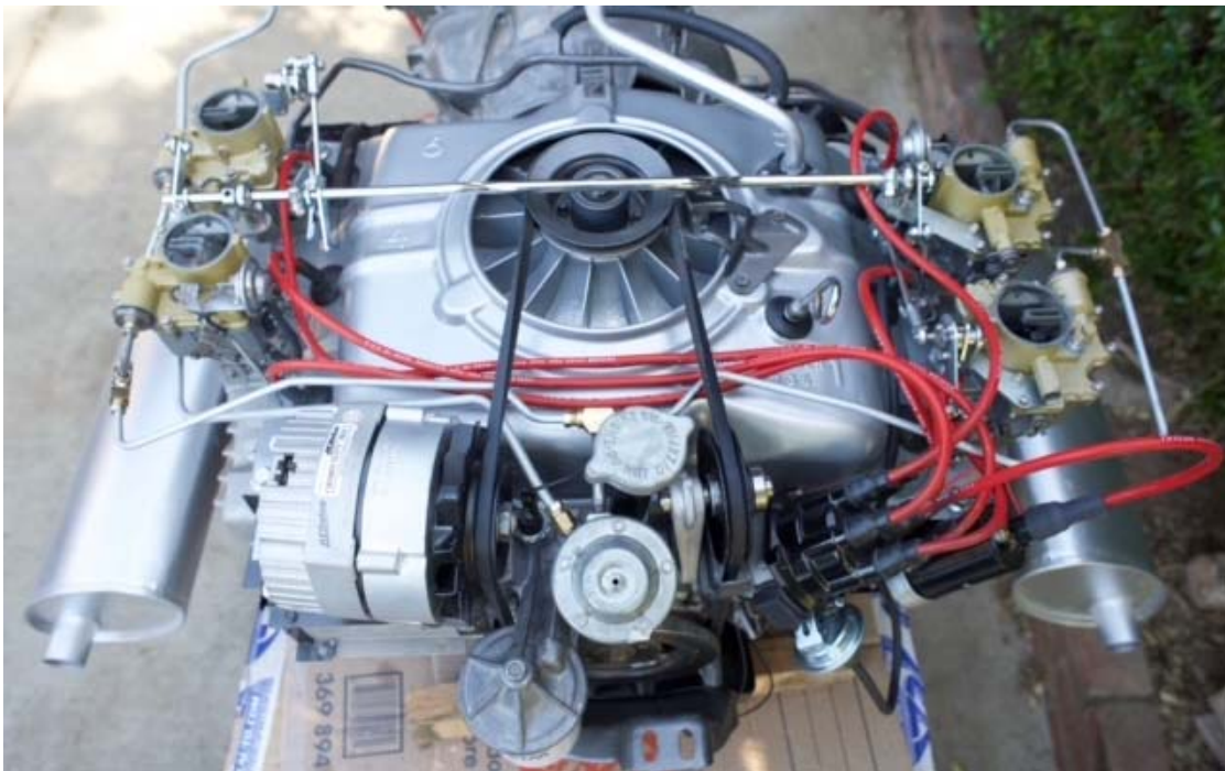
4-carb CORSA engine developing 140 HP, as used in 1965-66
